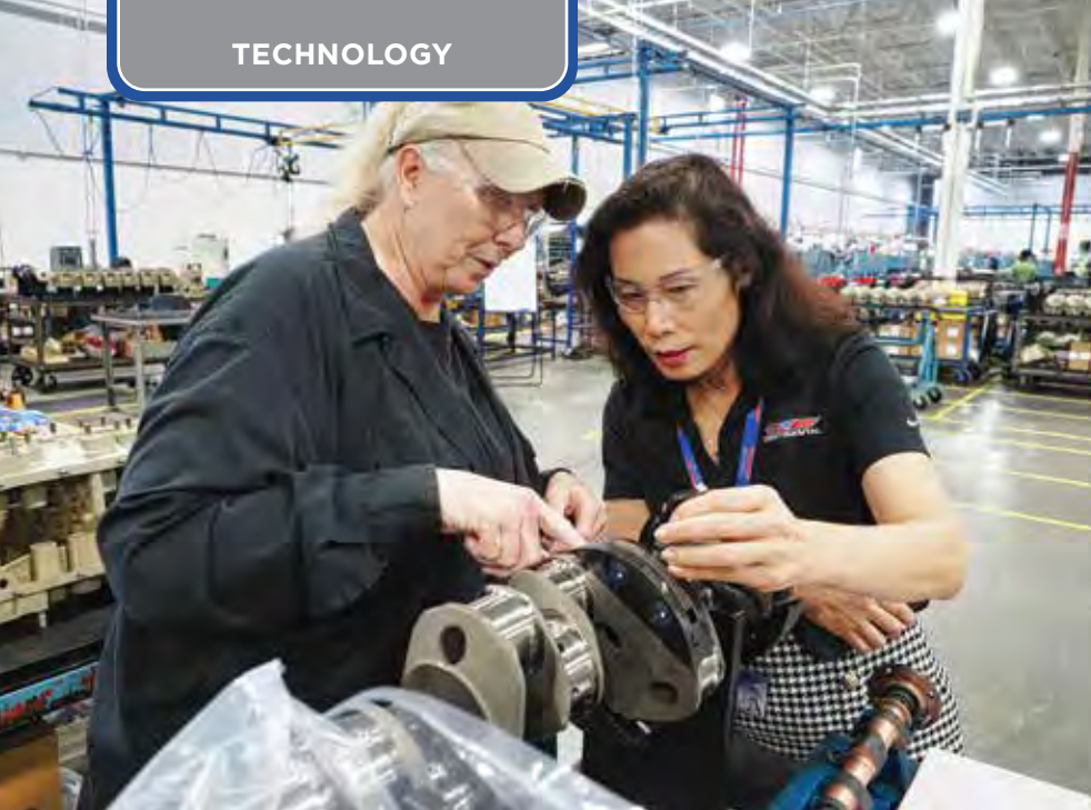
Carole Peterman (left), a quality team member, and Karen Hong, president and CEO of Continental Aerospace Technologies, carefully examine a crankshaft ahead of the engine assembly process.
